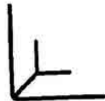
PVC CORNER MOULDING 007369 INTERNAL CORNER WHITE 007370 EXTERNAL CORNER WHITE 040149 INTERNAL CORNER SNOW WHITE For 4mm board, 2400mm length.
