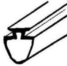
WEATHER SEAL-POP TOP EXTRUSION For aluminium pop top extrusion. Sold per metre. 007420
