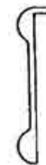
ALUMINIUM TABLE MOULD 25MM 035443 Flexible knock-in bead for trimming table and cabinet top edges. SPECIFICATIONS: • Dimensions: 25mm x 4000mm(L) • Mill finish
