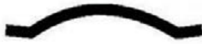
TRULINE INFILL MOULD Flexible PVC infill mould that locks into the Truline Aluminium extrusion to conceal fixing screws and rivets.
