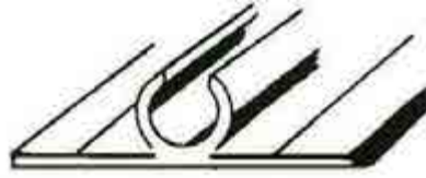
ROPE TRACK DOUBLE 042065 6.0M BLACK 042064 6.0M CLEAR ANODIZED 001649 6.5M BRIGHT WHITE Double fixing, aluminum track for securing vertical walls of annex.
